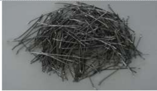
Figure No-3.1.1 Hooked End Steel Fibers
